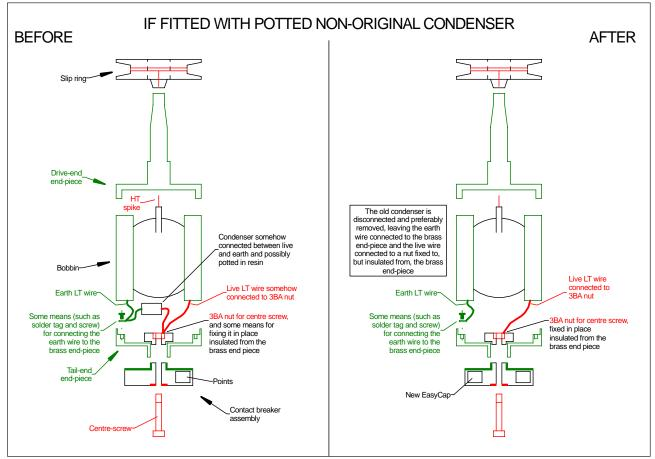
The C03 EasyCap is fitted to the contact breaker assembly between the two castings in place of the insulating plate(s) which should be removed.
