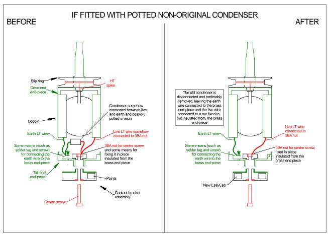
The C05 EasyCap is fitted between the two brass castings of the contact breaker assembly in place of the insulating plate(s) which should be removed.
