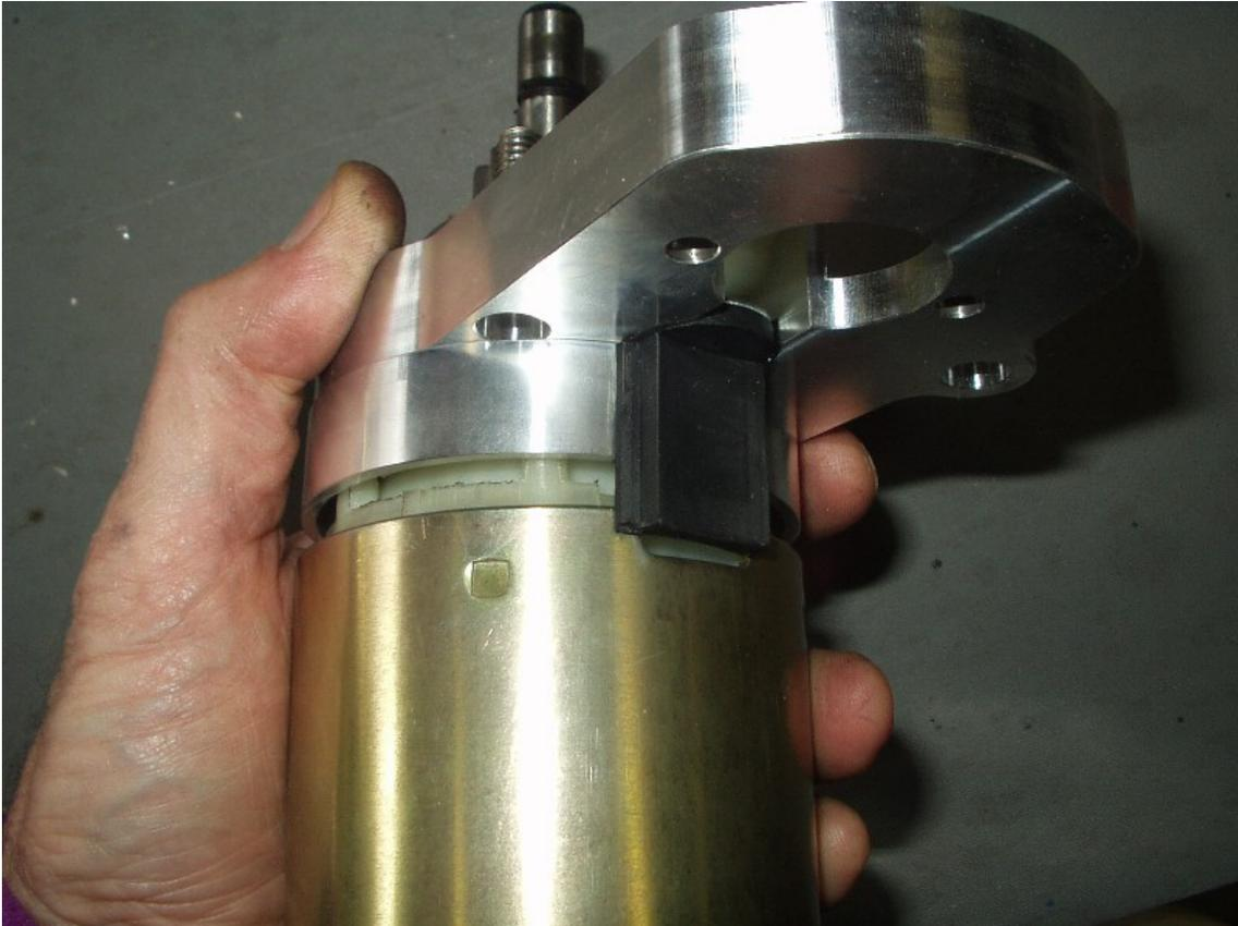
There is a steel ball that serves as a thrust bearing for the shaft inside the gearbox. Be sure that it does not fall into the planetary gears. The gearbox may come out with the motor. This is not a problem as the gearbox has to be removed from the motor anyway. The gearbox pulls straight off the end of the motor.
