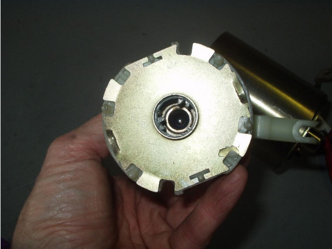
Push the armature and end plate out the end of the casing by pushing on the end of the motor shaft. Do not pull on the end plate or you will pull the brushes off the end of the armature. Getting the brushes back on the armature requires unbolting the brush plate from the end plate, inserting a thin ring to hold the brushes outward while re-inserting the armature. This is difficult to do without a holding ring.
