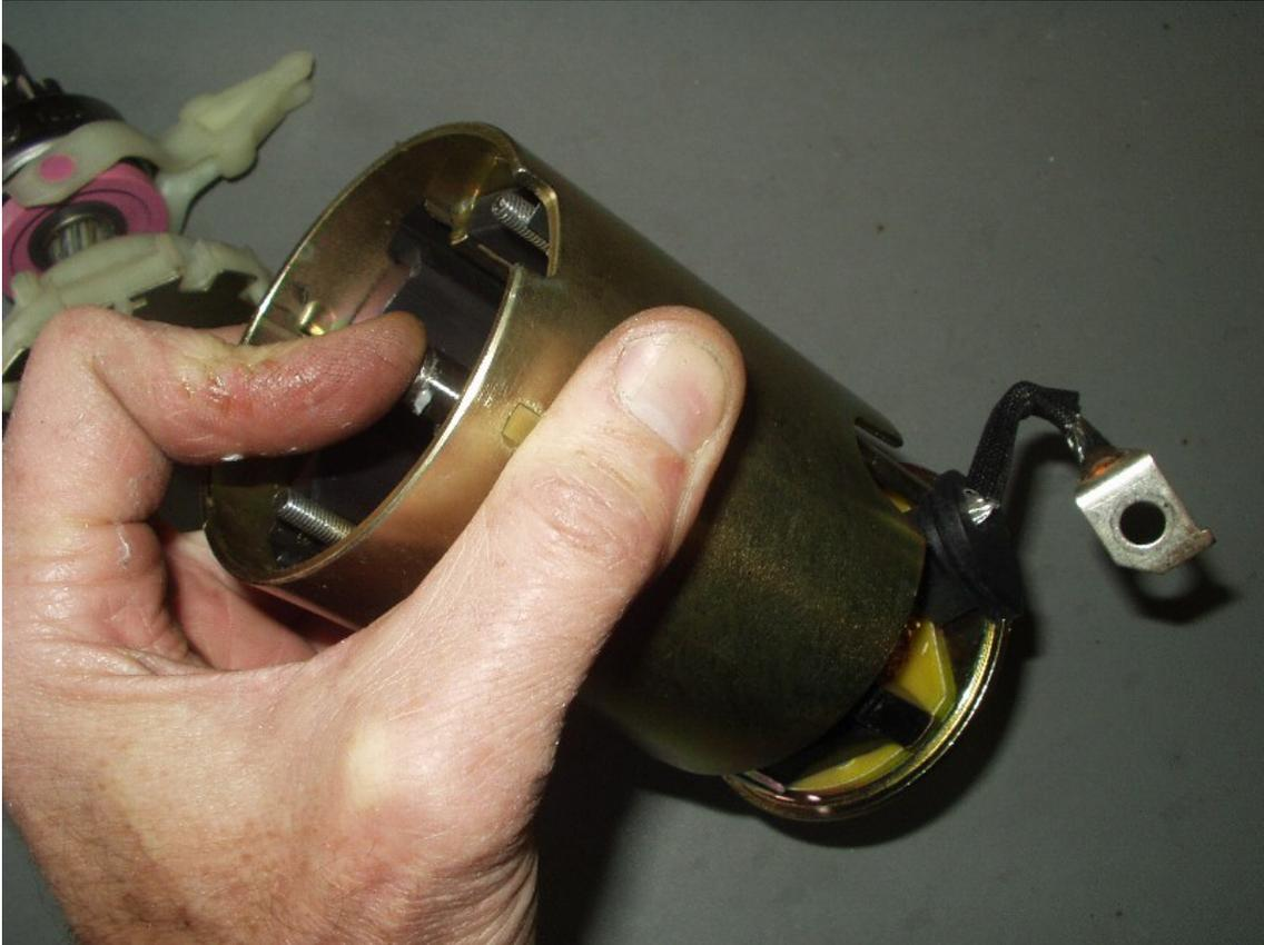
Set the armature and end plate aside. Using a pair of needle nose pliers, bend the magnet side of the spring clip tab on the brush end of the case just far enough to clear the magnets. Do not bend the spring clips too many times or they will break.
