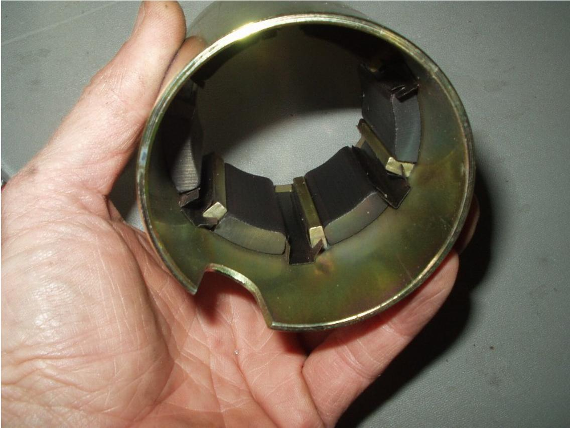
Mark each magnet in order. The magnets will be moved one place either clockwise or counter clockwise. I use the notch for the power wire as the #1 reference. Be sure the magnets do not jump onto each other or a steel plate. They are brittle and can break.
