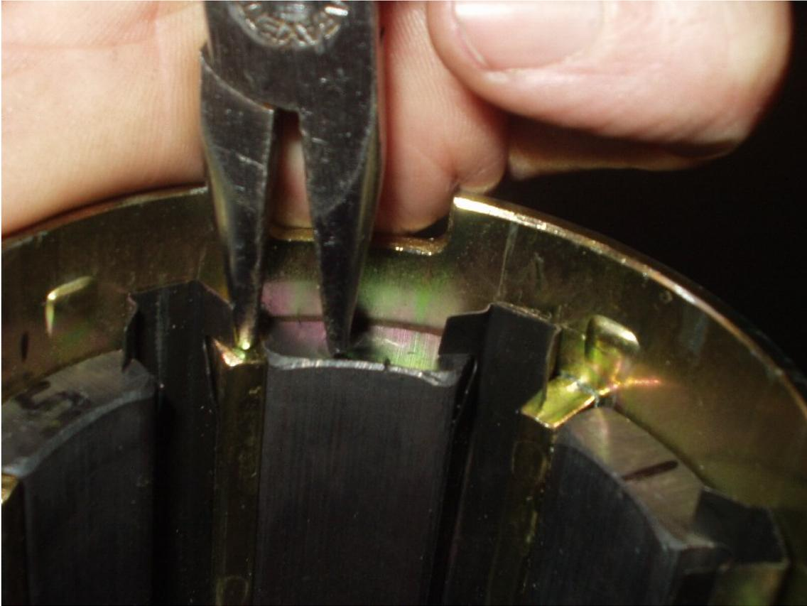
After the magnets are back in, bend the end of the spring clips back over the end of the magnets. The magnets are now one place around from their original positions.
