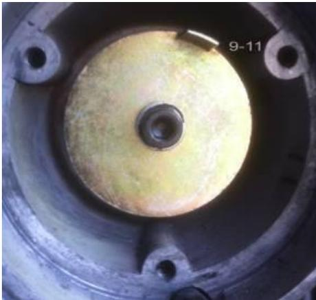
Fit the Tri-Spark rotor as shown here and tighten with the socket head cap screw and washer provided. There should be a 9 to 11mm gap between the right edge of the rotor tab and the casting as shown.
