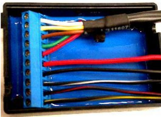
Connect the cable from the sensor plate to the control box as shown here. Also connect the wiring from the box to the ignition coils and wiring harness as shown in the following photo and wiring diagrams on page 6.
