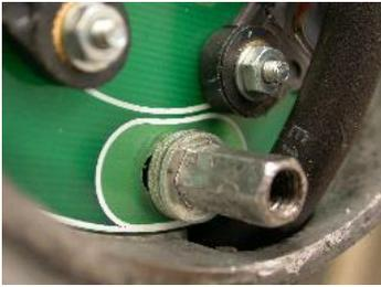
Fit the Sensor Plate using the original pillar bolts but do not tighten yet as it will be adjusted later during strobe timing. The positioning of the sensor plate is approximate at this stage as it will be adjusted later on when strobe timing. Use the LED as shown in step 6 to adjust the position of the sensor plate for more accuracy. You can do this after the wiring is connected in step 5.
