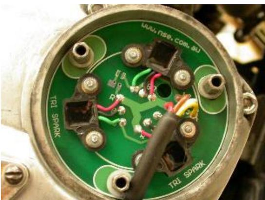
Feed the free end of the cable attached to the sensor plate through the hole in the bottom of the points cavity where the points wiring was originally located.
