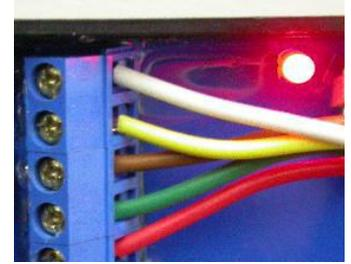
2 - Additionally, the LED can be used to check the sensor plate operation as follows. With the sensor plate removed from the engine to gain access to the sensors, a thin steel object inserted in the sensor slot should make the LED come on. It must be a steel object such as a hacksaw blade (not stainless steel or any other metal). This is an easy way to check that all 3 of the sensors are operating.
