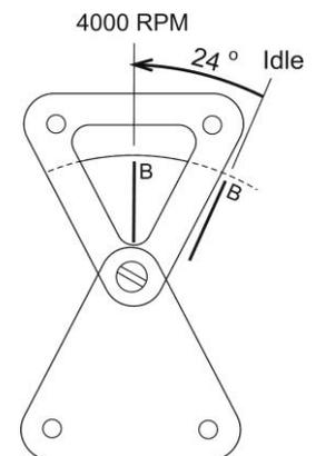
If required, the timing can be adjusted by rotating the sensor plate on its slotted holes. Moving the sensor plate anti-clockwise advances the ignition timing. If the adjustment slot range is insufficient to achieve the timing as described above, you may need to check and adjust the installation of the Tri-Spark rotor.
