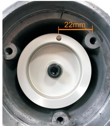
Important! Check that the face of the rotor is 2mm (+/- 0.6) below the deck that the stator sits on.
